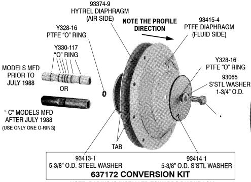
NOTE: RADIUS IS INSTALLED TOWARDS DIAPHRAGM
